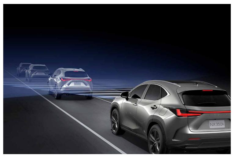
Pre-collision System (PCS) Vehicle Detection with Alarm Only - Stationary / Preceding Vehicle only
