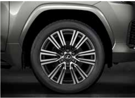
55.88cm (22 Inch) Wheels (265/50R22) Forged Aluminum wheels with Machined finish and Black Coating
